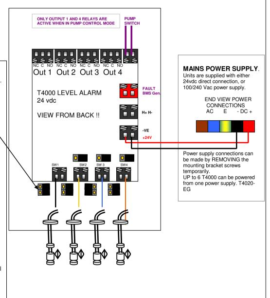
Description . T4000 STANDARD CONNECTING WIRING REQUIREMENTS DRG No T4000-STD WIRING
